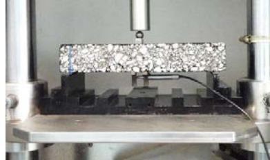
Fig. 2. Specimen during bending test mounted in Nottingham Asphalt Tester apparatus.
