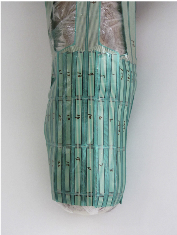
Fig. 1. Placement of sensors on residual limb.
