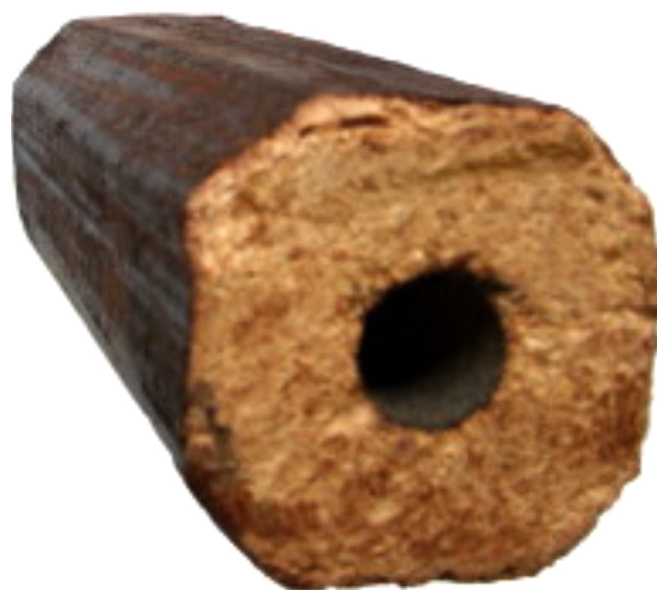
Fig. 13. Briquette with a concentric hole produced from a screw extruder/press. Used with permission by New-Air Technical Services Ltd. Leicester, England from [27].
