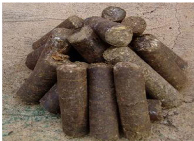
Fig. 8. Sugarcane bagasse briquettes from a hydraulic press. From [62]. Used with permission.
