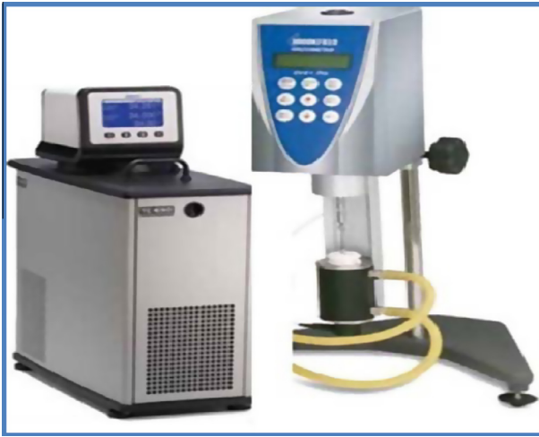
Figure 3 Brookfield Viscometer DV + II type with water bath TC-650.
