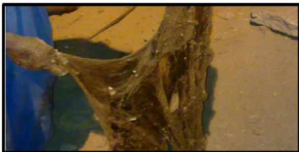
Figure 8 The gummy shape of crude oil treated with a high concentration of DRA.
