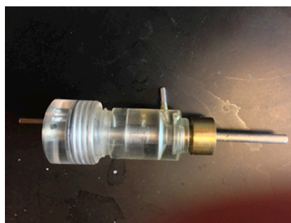
Hydraulic microelectrode advancer made by David Hubel
