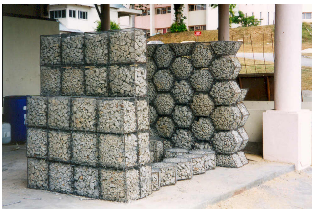
Figure 3 Different types of wall gabions constructed for the test model.
