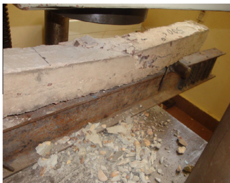
Fig. 7 Failure mode of unprotected RC beams after 2-h exposure to 500 and 600 °C.
