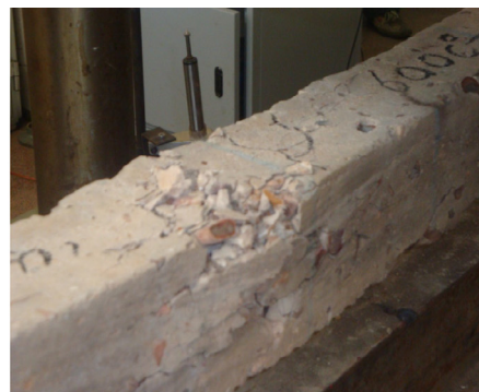
Fig. 7 Failure mode of unprotected RC beams after 2-h exposure to 500 and 600 °C.
