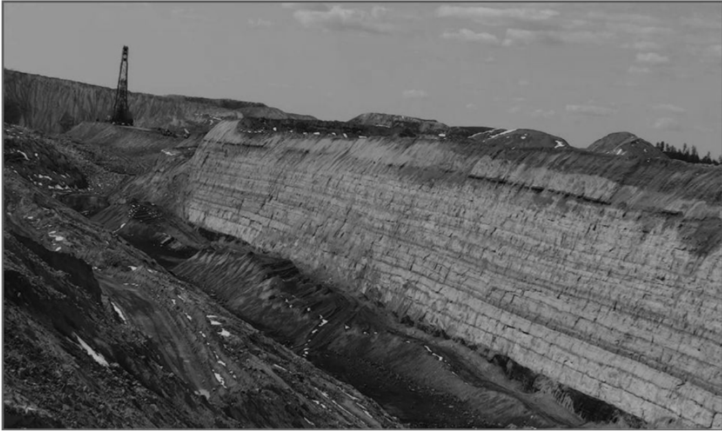
Fig. 7 : Open pit casting operation of 150' (45M) face.
