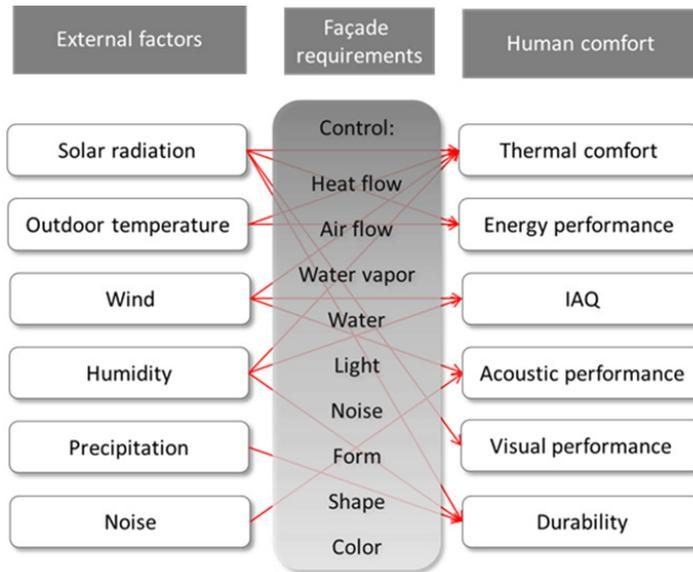
Fig. 3. Schematic role of adaptive façade.
