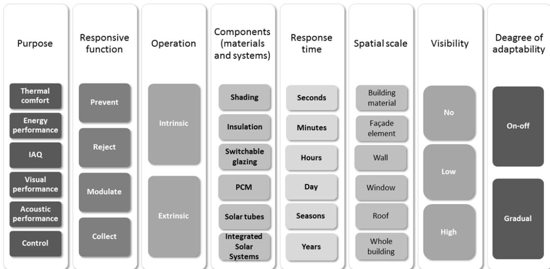
Fig. 2. Overview of characterization concepts for envelope adaptivity. Adapted from [10]
