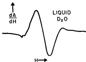
FIGURE 1 NMR spectrum of liquid  $D_2O$ . 3 ml of 99.7% pure liquid  $D_2O$  at a temperature of approximately  $20^\circ C$  was used. The NMR spectrum was recorded as a plot of  $dA/dH$  (the derivative of radio frequency absorption with respect to magnetic field) vs.  $H$  (magnetic field strength). The peak-peak width of this spectrum was estimated at approximately  $60 \pm 30 \times 10^{-3}$  gauss.
