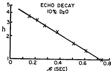
FIGURE 4 Echo decay for 10% D<sub>2</sub>O. Sample was 2 ml of 10% D<sub>2</sub>O-90% H<sub>2</sub>O in air at 24.5 C. Height ( $h$ ) of the echo following the 90°-180° pulse pattern was measured as a function of time ( $t$ ) between the echo and the 90° pulse.  $h$  is expressed in arbitrary units.  $h$  on a log scale is plotted against  $t$ . From the line drawn through the data points,  $T_2$  is estimated to be 0.45 sec, which is the time for  $h$  to decay to 1/e of a previous value.
