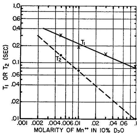
FIGURE 6  $T_1$  and  $T_2$  vs.  $[Mn^{++}]$  in D<sub>2</sub>O. Various concentrations of MnCl<sub>2</sub> are dissolved in 10% D<sub>2</sub>O-90% H<sub>2</sub>O.  $T = 25^\circ \pm 1^\circ C$ .
