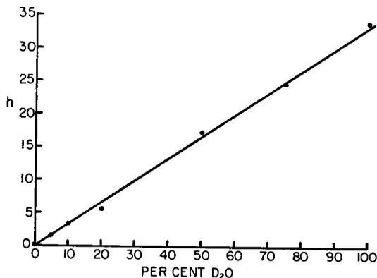
FIGURE 2 Standard curve for analysis of  $D_2O$  in  $H_2O$ . Mixtures of  $D_2O$  in  $H_2O$  were made up as per cent by volume and were analyzed for D by NMR at  $20^\circ C$ . On the abscissa is plotted per cent  $D_2O$ . On the ordinate,  $h$  represents the peak-to-peak height of the NMR spectrum measured for the sample, divided by the voltage gain of the output amplifier of the NMR spectrometer. Each point represents the mean of two NMR spectra on the same sample.
