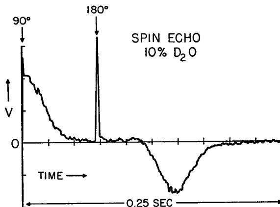
FIGURE 3 Free induction decay and echo of deuterium in 10%  $D_2O$ -90%  $H_2O$  at 24°C. Sample volume is 8 ml. Voltage ( $V$ ) output of the phase detector is plotted against time. The sample is subjected to the  $90^\circ$  pulse ( $1 \times 10^{-3}$  sec duration) at zero time, which is followed by emission by the sample of a free induction decay, after which the sample is subjected to a  $180^\circ$  pulse ( $2 \times 10^{-3}$  sec). The echo is emitted by the sample at an equal time later.
