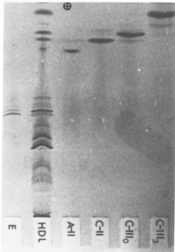
Fig.3. Analysis of rat apo C-II, C-III and A-II fractions obtained by preparative isoelectric focussing of apo HDL (fig.1) by analytical polyacrylamide slab-gel isoelectric focussing in a pH 4–6 gradient [16]. Apo E was prepared from delipidated [16] rat VLDL by preparative isoelectric focussing as in fig.1.
