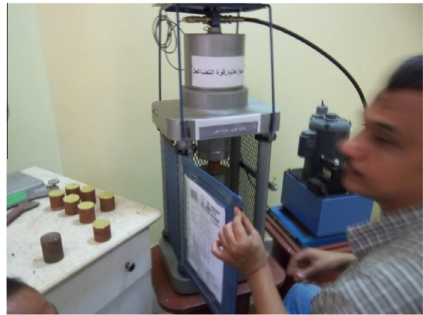
Figure 8 Compressive strength test for core of concrete sample.
