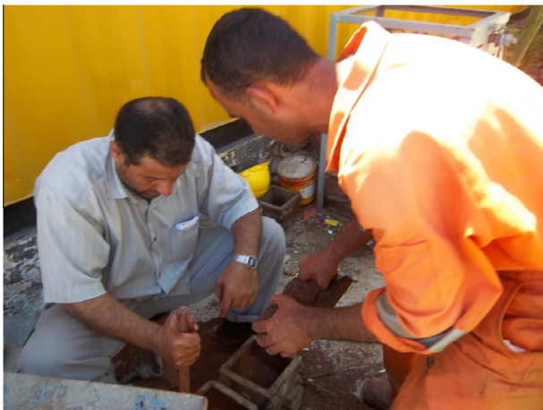
Figure 7 Preparing cubic samples for compressive strength of concrete to test.
