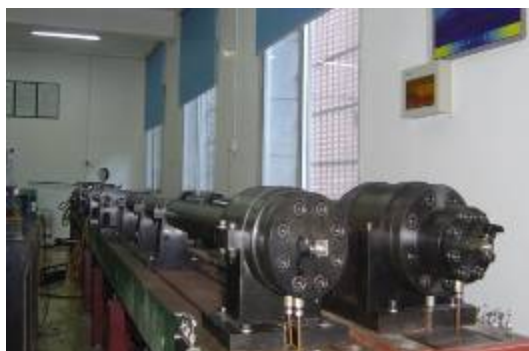
Fig.3 SHPB system for rock testing with coupled loads.
