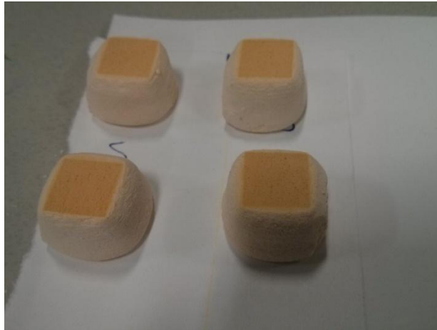
Figure 3: Parts after curing for 2.30 hour at 200°C
