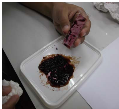
Fig. 7. Condition of electrode when soak in dye of fruit
