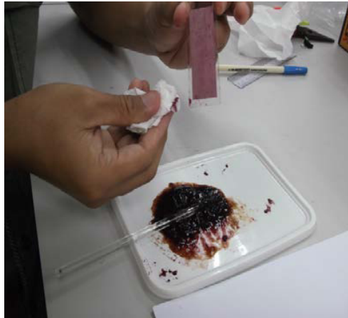
Fig. 8. Remove the stained electrode and clean it carefully with tissue
