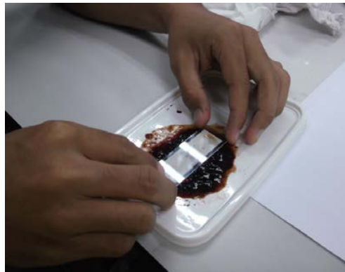
Fig. 6. Slowly immerse the sintered titania electrode in the staining
