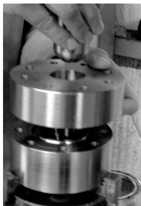
Fig. 2. The punch, die and die cap used for measuring the FLC.
