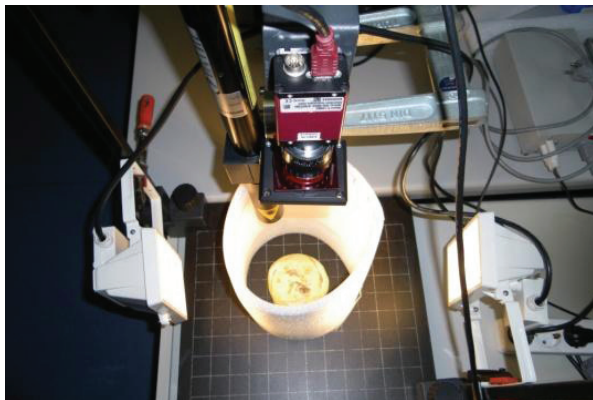
Fig. 3. Experiments with a monochrome camera with different optical band-pass filters
