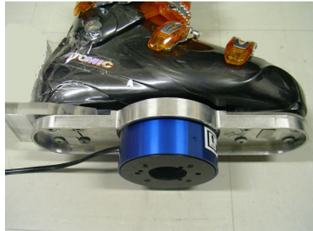
Fig. 2. Measurement system of reaction force from snow surface
