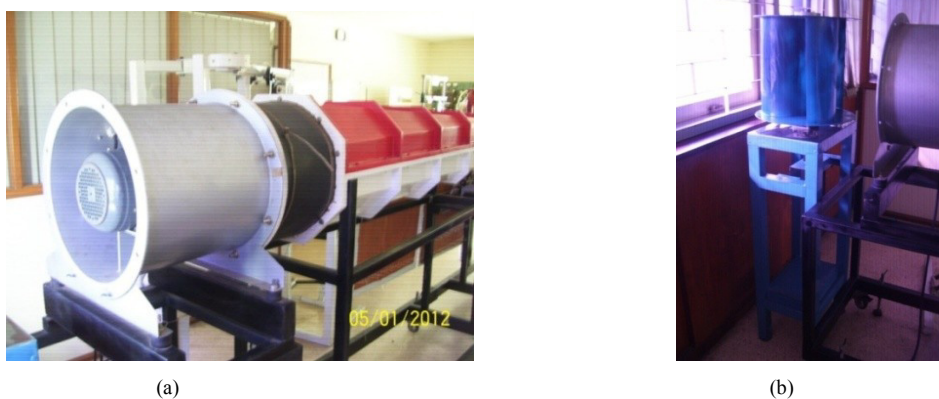
Fig. 6. (a) Wind tunnel, and (b) Savonius wind turbine model.
