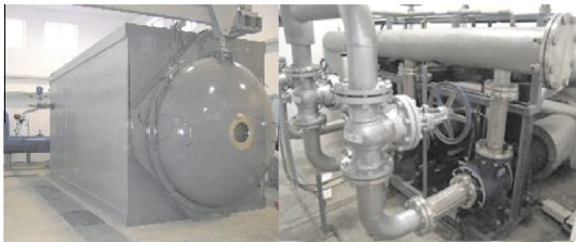
Fig. 1 Large multi-parameter environmental simulation test cabin.
