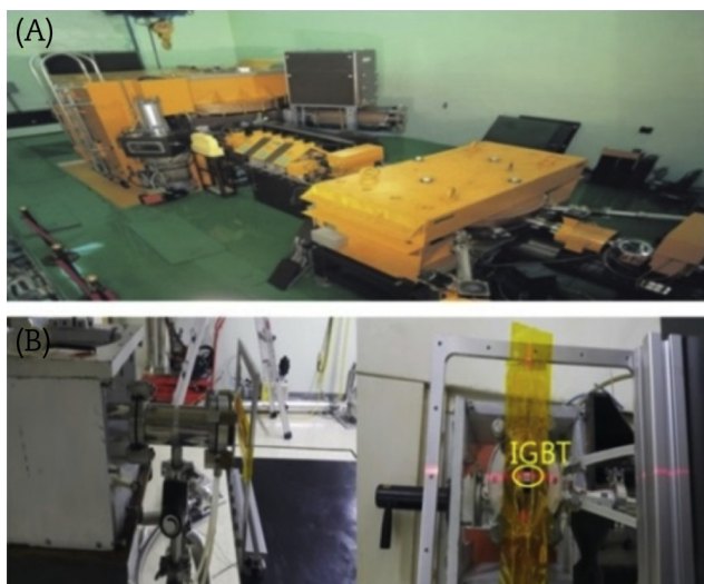
Fig. 2 – MC-50 cyclotron at Korea Institute of Radiological and Medical Sciences. (A) MC-50 cyclotron. (B) Sample mounting at the end of beam line #2.
