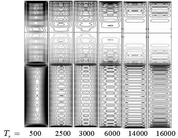
Fig. 4. Stream lines of the Secondary Flow (top) and contours plot of Axial flow (bottom) in each row at Dean number ( $D_n$ ) = 1000 and  $M_g = 5000$  for Flux ( $Q$ ) versus Taylor number ( $T_r$ ) at  $T_r = 500, 2500, 3000, 6000, 14000$  and  $16000$  .
