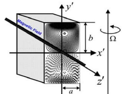
Figure 1: Co-ordinate system in a Rotating Straight Duct
