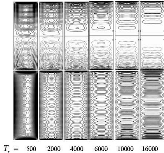
Fig. 6. Stream lines of the Secondary Flow (top) and contours plot of Axial flow (bottom) in each row at Dean number ( $D_n$ ) = 2000 and  $M_g = 5000$  for Flux ( $Q$ ) versus Taylor number ( $T_r$ ) at  $T_r = 500, 2000, 4000, 6000, 10000$  and  $16000$  .
