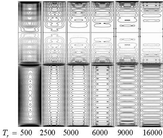
Fig. 3. Stream lines of the Secondary Flow (top) and contours plot of Axial flow (bottom) in each row at Dean number ( $D_n$ ) = 500 and  $M_g = 5000$  for Flux ( $Q$ ) versus Taylor number ( $T_r$ ) at  $T_r = 500, 2500, 5000, 6500, 9000$  and  $16000$  .
