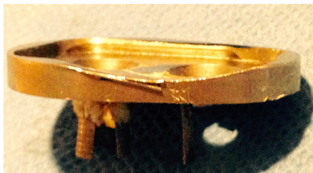
Fig. 4. Wear on the posterior side of the metal glenoid baseplate due to metal-on-metal contact with the humeral head.
