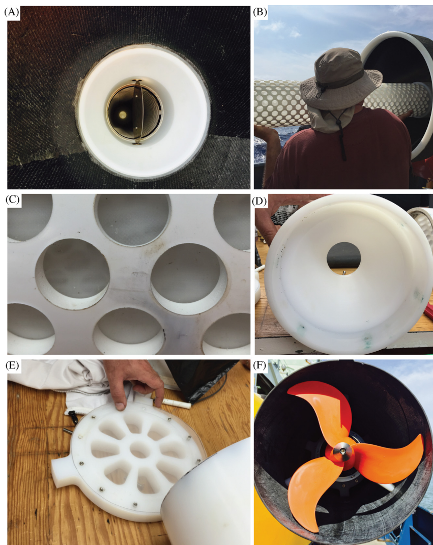
Fig. 4. SyPRID components. (A) In-line valve, (B) filter, (C) filter detail, (D) cod end, (E) sample mesh, and (F) axial flow pump.
