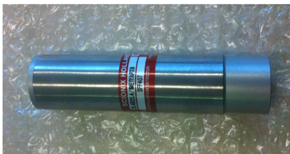
Fig. 2. Photograph of a YAP(Ce) detector. A cylindrical 1 in. long by 1 in. in diameter crystal (right) was coupled to 1 in. diameter PMT. Figure from Ref. [7].
