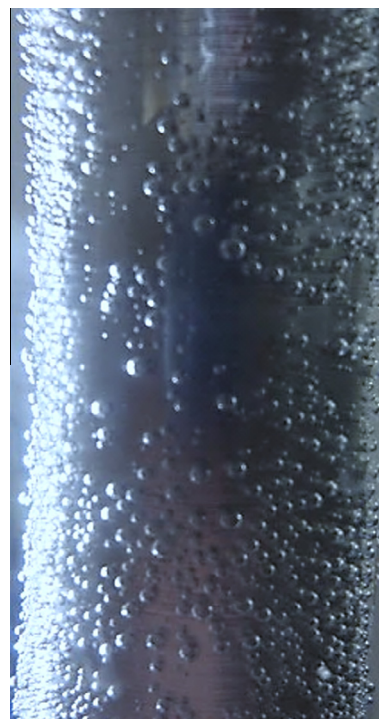
Figure 16 Bubble formation at heat flux (a) 45 \text{ kW/m}^2 , (b) 54 \text{ kW/m}^2 , (c) 63 \text{ kW/m}^2 , (d) 91 \text{ kW/m}^2 , (e) 110 \text{ kW/m}^2 , and (f) 132 \text{ kW/m}^2 .
