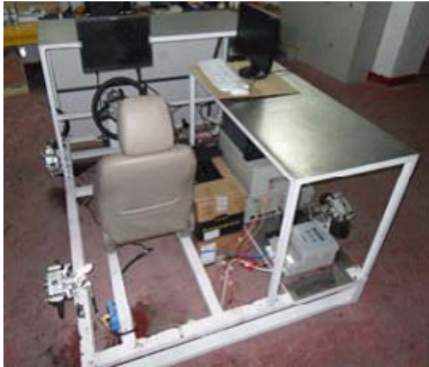
Fig. 1. HIL test bench of traction control system
