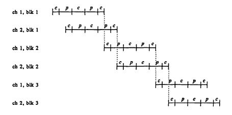
Figure 1. Pipelined execution of two-dimensional FFT yielding 100% utilization of processing and communications. Notation: c denotes a communications stage; p denotes a processing stage; (ch i, blk j) denotes block j of channel i.
