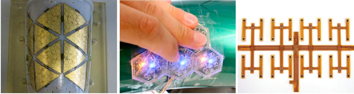
Fig. 1. Different robot skin technologies in [14] (left), [12] (middle) and [8] (right). In the left image, capacitive transducers are used to provide tactile feedback, and are placed on flexible PCB. In the middle image, rigid but small multi-modal modules sense touch, temperature and vibration. In the right image, touch sensors are placed on foldable modules.
