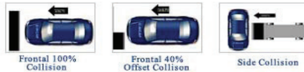
Fig.2. Schematic Diagram Of C-NCAP Crash Test Program
