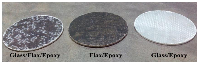
Fig. 3. Sound test specimens
