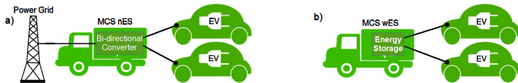
Fig. 2. MCS working mode; (a) on-grid charging mode; (b) off-grid charging mode.
