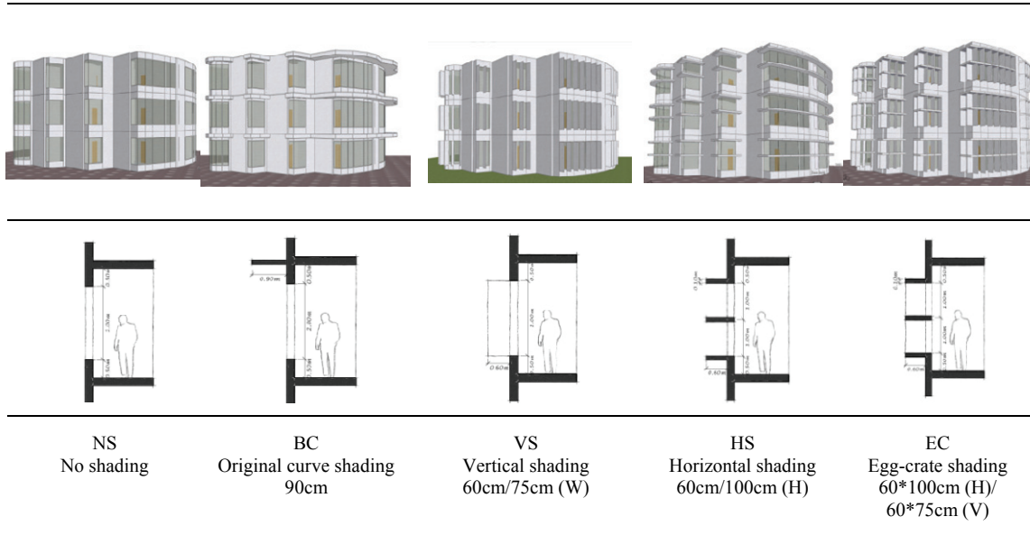
Fig. 3. The alternative designs for the three types of shading devices (Source: Author)
