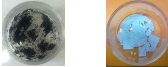
Figure 5 Pictures of PVDF (left) and Nylon (right) membranes after 2 months operated under protocol D conditions.
