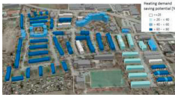
Figure 5 – Heating energy saving potential, visualised in the 3D city model Grünbühl
