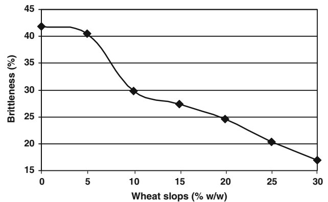
Fig. 2 Dependence between brittleness of rigid PUR-PIR foams and content of solid fraction of wheat slops
