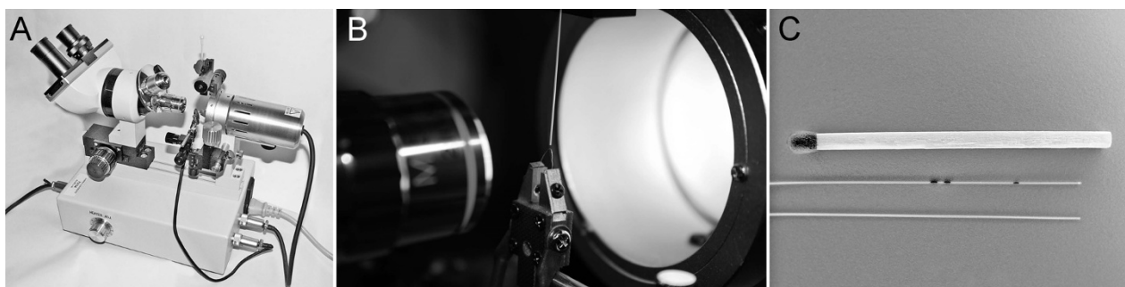
Figure 1 Manufacturing of the occluding filaments. A shows the MF-830 micro forge (Narishige Scientific Instrument Laboratory, Tokyo, Japan) used for the manufacturing of the occluding filaments. The tip of the microloader (Eppendorf AG, Hamburg, Germany) was positioned just above the heatable platinum wire as shown in B . The rounded tip was formed by increasing the temperature of the platinum wire. The heating process was activated and controlled with a foot pedal and could simultaneously be followed through the oculars of the micro forge. The microloader with the black marks has a rounded tip, whereas the microloader below has not been modified ( C ). The marks were used for the correct positioning of the microloader in the internal carotid artery. The last black mark was placed 22 mm behind the rounded tip and had to be positioned on the level of the carotid bifurcation.
