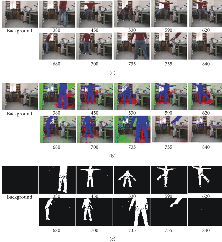
FIGURE 9: The results of foreground detection, (a) original images, (b) the results of pixel classification, where the red color indicates the shadow, green indicates the highlight, and blue indicates the foreground, (c) the results of background subtraction with shadow removal using our proposed method, where dark indicates the background and white indicates the foreground.
