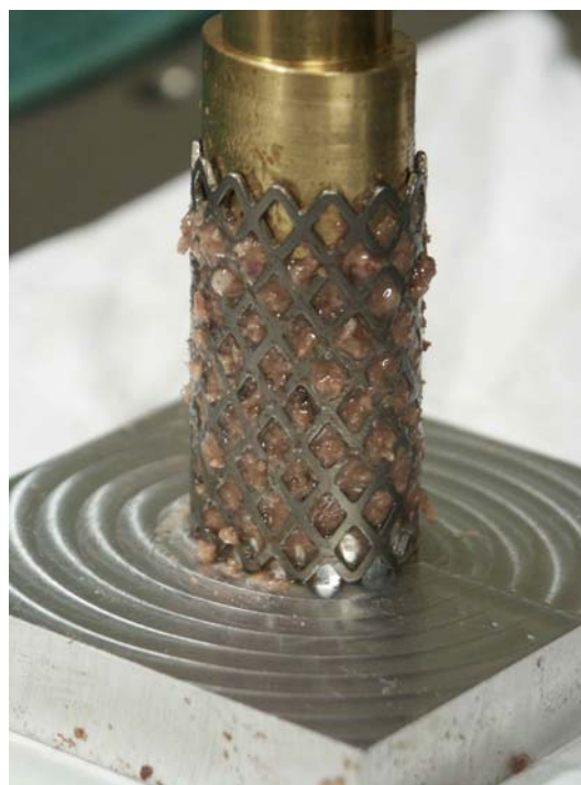
Fig. 2 Harms cage filled with bone graft in a contained and loaded condition
