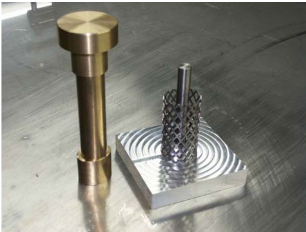
Fig. 6 Impactor and Harms cage with a central nail
