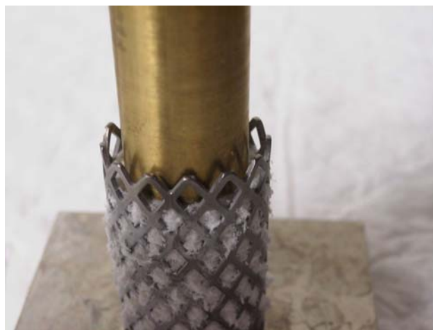
Fig. 4 Mismatch between Harms cage and cylindrical plunger leading to un-containment
