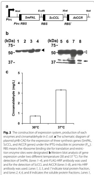
2, 5, and 6 indicate samples at 30 °C, and *lanes 3, 4, 7,* and 8 indicate samples at 37 °C. Symbols: *Closed arrowhead*, SmPAL; *open arrowhead*, ScCCL; *solid arrow*, AtCCR. **c** HPLC analysis of cinnamaldehyde produced under two different temperatures. *Error bars* represent standard deviation of the mean (n = 3)
