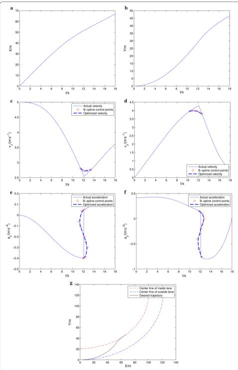
**Fig. 6** Desired trajectory, velocity and acceleration. **a** X-axis displacement, **b** Y-axis displacement, **c** X-axis velocity, **d** Y-axis velocity, **e** X-axis acceleration, **f** Y-axis acceleration, **g** desired trajectory
