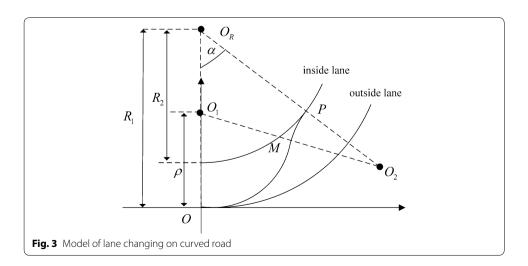
$O_1$  and  $O_2$  respectively. These two arcs are tangent in M,  $\alpha$  is the rotation angel between  $OO_R$  and  $PO_R$ .
