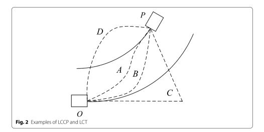
O o D o P, the extremum of curvature appears in the starting position. It does not meet the LCCP *Constraint 2*. O o A o P and O o B o P are the paths that can be achieved in practice. These two paths can satisfy the LCCP constraints. In addition, there are a great many other paths which can satisfy the LCCP constraints. In this paper, we mainly research the paths composed of two segments arcs which like O o A o P.
