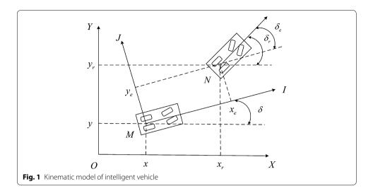
where  $A(q) = \begin{bmatrix} \sin \delta - \cos \delta & 0 \end{bmatrix}$  is a vector associated with non-holonomic constraints,  $\dot{q} = \begin{bmatrix} \dot{x} & \dot{y} & \dot{\delta} \end{bmatrix}^T$ . On this basis, the kinematic model equation is established (Kanayama et al. 1990)
