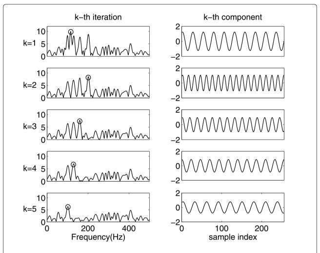
**Figure 3 Five iterations of the MP for a noisy signal**. The left column shows each iteration of the MP and the selected component is marked by a open circles; the right column shows the corresponding signal component extracted at each iteration.
