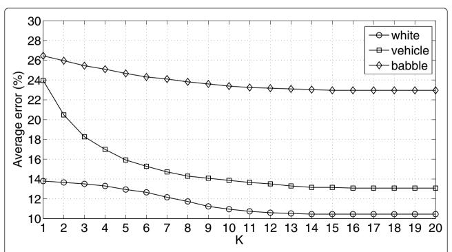
Figure 7 Average error for speech detection when increasing the iteration number K in the atomic decomposition in white, vehicle, and babble noise (SNR = 0 dB).
