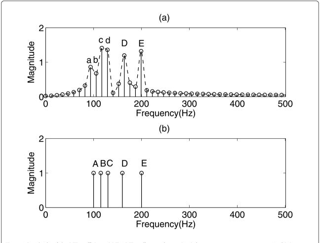
Figure 1 Drawbacks of the DFT coefficients. (a) The DFT coefficients of a signal with frequencies: 100, 115, 130, 160, 200 Hz; (b) the accurate frequency components of the signal.
