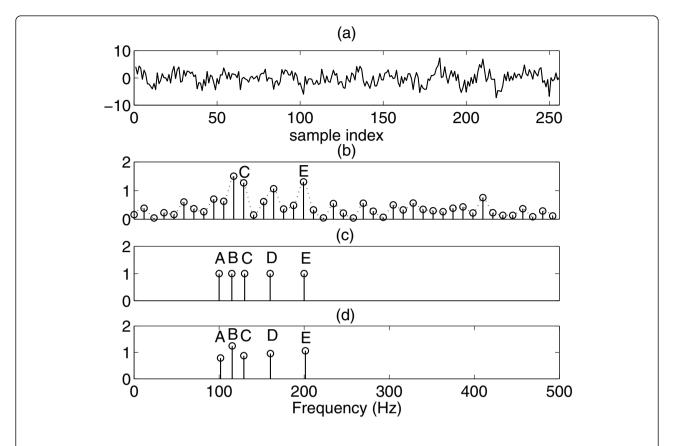
**Figure 2 Decomposition of a noisy signal by DFT and the conjugate subspace MP. (a)** The noisy signal; **(b)** the DFT coefficients of the noisy signal; **(c)** the accurate frequency components of the original signal; **(d)** the MP coefficients of the noisy signal after five iterations.
