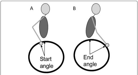
**Figure 2 Definitions of start angle and end angle.** (A) The start angle is the angle between the line which connects the initial hand-rim contact point of the propulsion phase to the wheel center and the vertical line. (B) The end angle is the angle between the line which connects the final hand-rim contact point of the propulsion phase to the wheel center and the vertical line.
