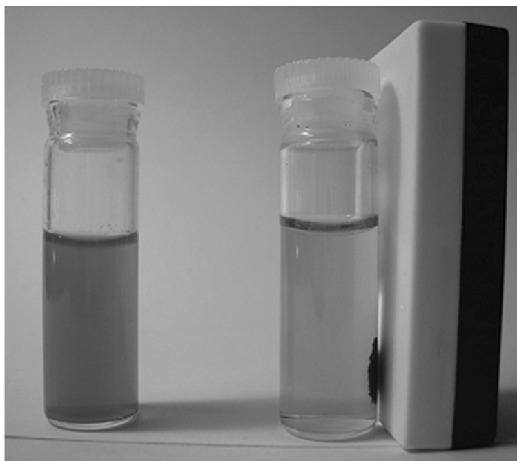
Figure 3 Magnetite-hexane suspension attached to a magnet.
