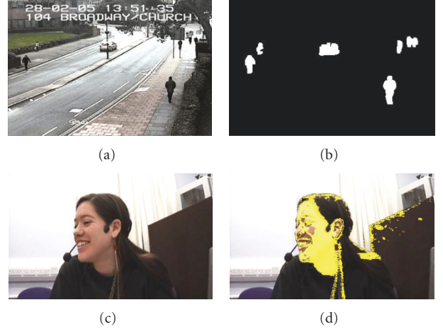
FIGURE 4: Sample segmentation results on CLEAR test sequences. (a) Outdoor test sequence and (b) corresponding motion segmentation result. (c) Indoor test sequence and (d) corresponding color segmentation result.
