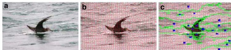
Figure 4 An example of extracting superpixels and heat sources from an input image. (a) The input image, (b) the superpixels extracted by Turbopixels [14] are encircled with red boundaries, and (c) the regions extracted by an agglomerative clustering scheme are encircled with green boundaries, and the extracted heat sources are colored in blue.
