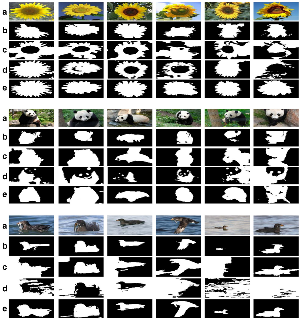
Figure 5 Segmentation comparison with ClassCut [9], Joulin et al. [19] and CoSand [4] on the Oxford flowers, UCSD birds and CMU iCoseg datasets. The regions in white indicate the foreground objects, while the regions in black stand for the backgrounds. (a) The input images, (b) ClassCut [9]’s results, (c) Joulin et al. [19]’s results, (d) CoSand [4]’s results, and (e) our method’s results.
