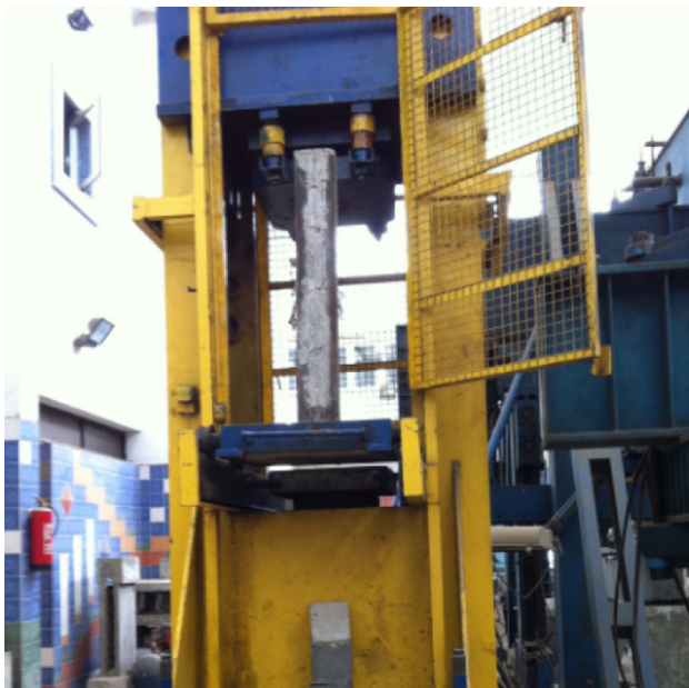
Fig. 5 Experimental testing machine of strengthened columns
