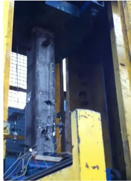
Fig. 6 Instrument for testing the strengthened RC columns with steel angles and strips
