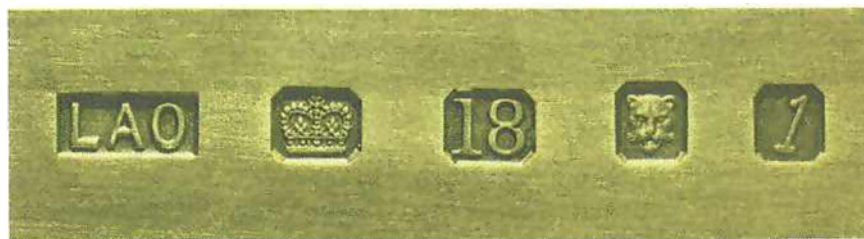
A set of hall-marks on a piece of gold plate. First comes the maker's mark, ordained in 1363 by Edward III, followed by the standard marks for gold, the crown with the 18 carat mark, then the leopard's head, established by Edward I in 1299, and finally the date letter, in this case for 1966. Date letters were introduced just 500 years ago in 1478
