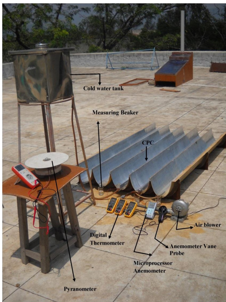
Figure 4 Pictorial view of air blower arrangement.
