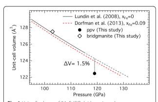
**Fig. 1** Unit cell volumes of (Mg,Fe)SiO $_3$  bridgmanite and ppv versus pressure. The unit cell volumes of the Fe-depleted bridgmanite at 102.5 GPa and the ppv phase at 119 GPa coexisting with the H-phase are compared with the equations of state for Fe-free MgSiO $_3$  bridgmanite (Lundin et al. 2008) and (Mg $_{091}$ Fe $_{009}$ )SiO $_3$  bridgmanite (Dorfman et al. 2013)
